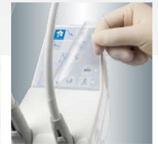
Disposable covers for dentist's and assistant's control panels. On the Full Touch version a special key temporarily deactivates the touch-sensitive screen to allow cleaning without interfering with the controls.
