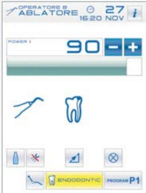
In addition to viewing data, the dentist can also set numerous work parameters: spray mode, foot control mode, optic fibre on/off. The control panel can also be used to personalise parameters for up to three different users, while parameters for a fourth user can be loaded via a USB memory device.
