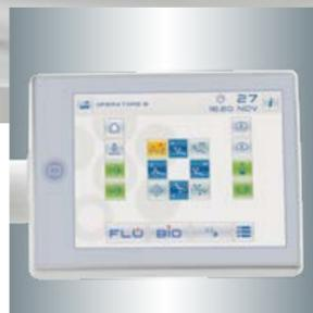
The accelerometer on the instrument control panel also allows the screen to be positioned horizontally.
