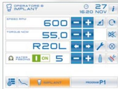
The i-XS4 micromotor electronic controls include speed, torque, plus delivery rate/operation of the peristaltic pump. Personalised settings are available for execution of the guide hole, the drilling stages and implant placement.
